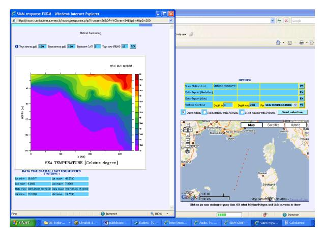
Using "Select station with polyline" it is possible to select stations. After clicking on Send selection, they will be viewed in the Google map. It is possible to select a vertical interval, a parameter and click on VC button. A section map will be produced.
