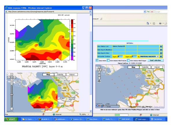
"Select station with polygon" allows the selection of a polygonal area. All station inside the polygon are selected (Send selection). User can choose the depth interval and the parameter to be mapped and clink on HC (Horizontal contour). The horizontal map is overlayed on a Google map. The user can change the parameters of interpolation.
